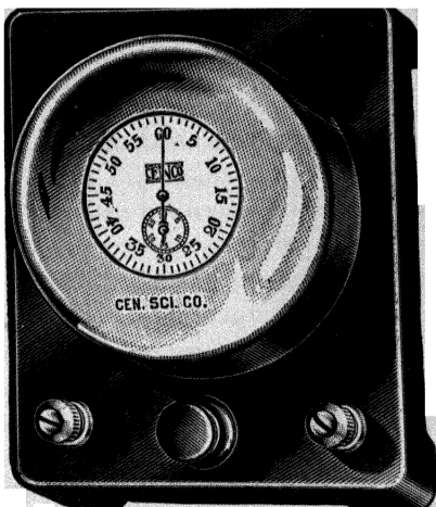
FIG. 16a.—Electric vibrator for measuring small intervals of time.
