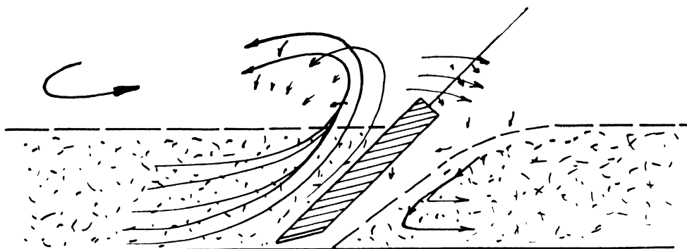
FIG. 140.—DIAGRAM SHOWING THE FORCING UPWARDS AND OVER OF AGGREGATE IN AN EIRICH PAN
