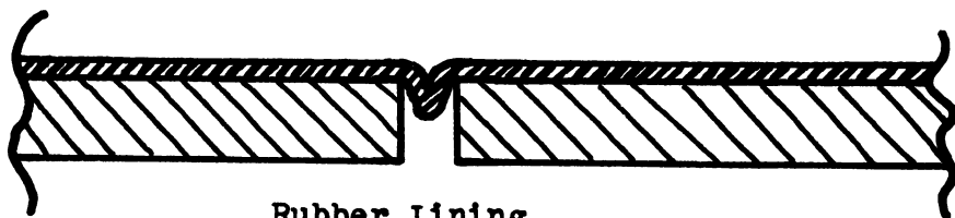
Rubber Lining on Unprotected Seam
