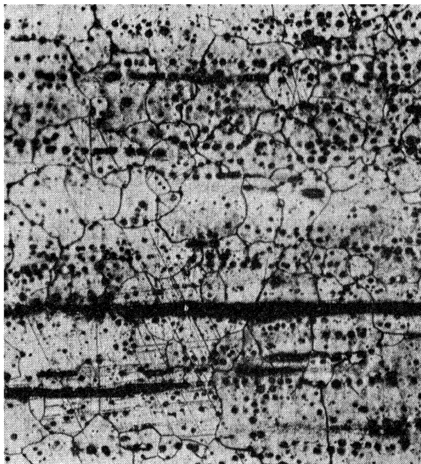
FIG. IV-17.—WROUGHT IRON (SHOWING SLAG INCLUSION).
