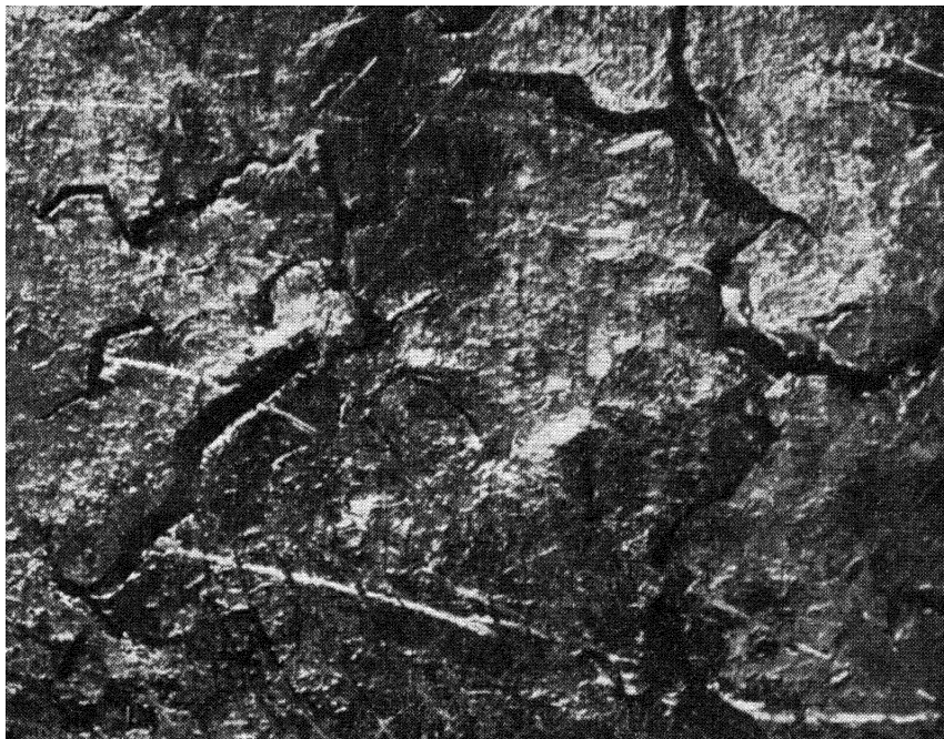
FIG. VI-7.—CORROSION CRACKING OF LEAD.
