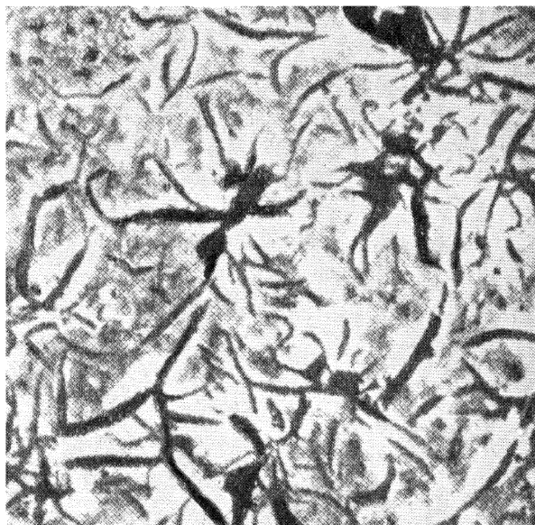
FIG. III-7.—GREY CAST IRON, SHOWING COARSE GRAPHITE.
