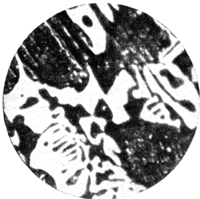
FIG. III-6.—WHITE CAST IRON. CEMENTITE (LIGHT), PEARLITE (DARK).
