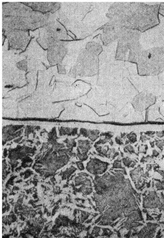
FIG. IX-1.—PHOTO-MICROGRAPH OF NICKEL-CLAD STEEL.
