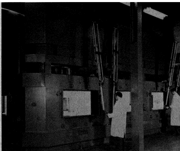
Figure 2. Three cell intermediate level metallurgy cave for 100 curies
