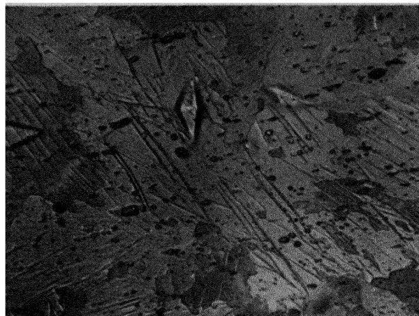
Figure 12. Microstructure of irradiated uranium obtained from aluminized plastic replica by metallographic microscope under inactive conditions; X240
