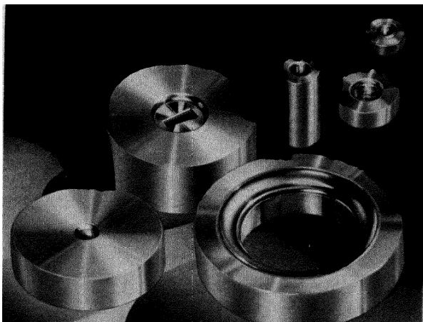
Fig. 358. Forming, sizing, and calipering dies with cemented carbide liners (courtesy of A. C. Wickman Ltd.).
