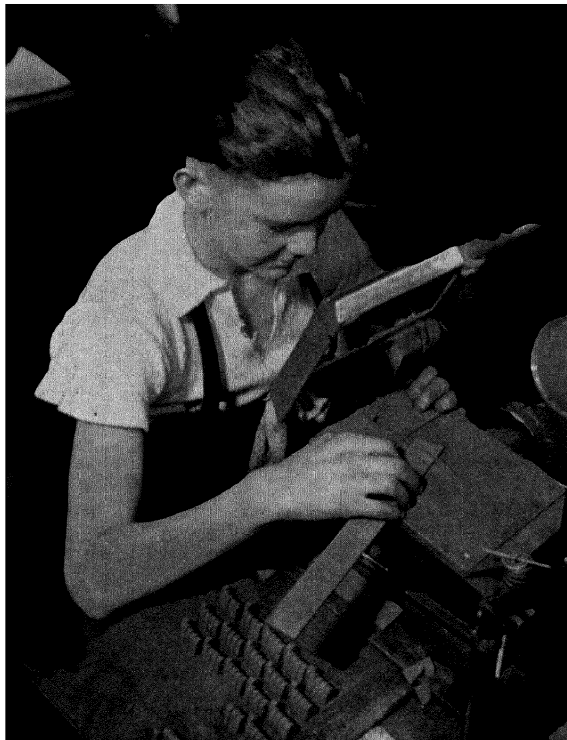
Fig. 337. Forming of presintered tungsten carbide slabs into the shape of small tool tips by means of a diamond saw (courtesy of A. C. Wickman, Ltd. and The Hydraulic Press Manufacturing Co.).
