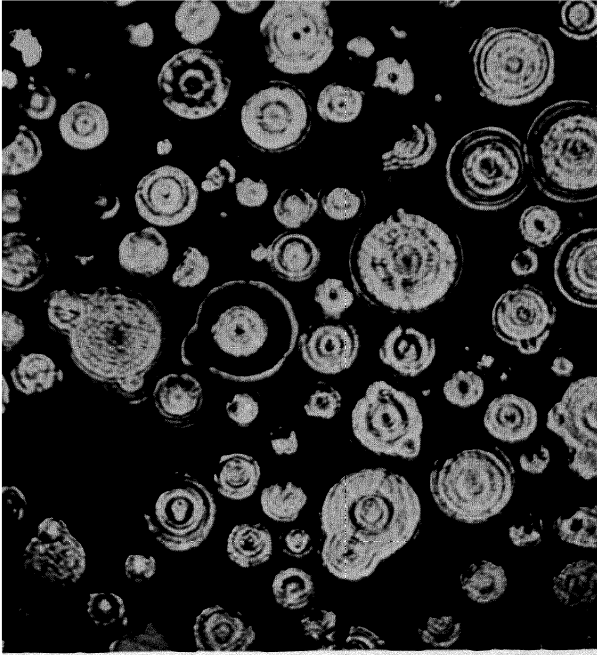
Fig. 429. Sectioned carbonyl iron powder (type "E") showing specific "shell structure" of each individual particle (courtesy of General Aniline Works).
