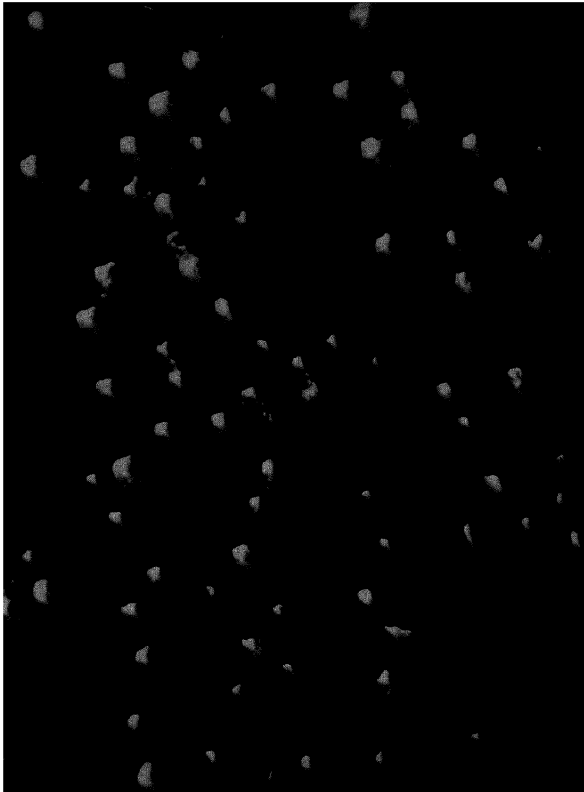
Fig. 562. Surface appearance ( \times 10 ) of spherical copper powder (courtesy New Jersey Zinc Co.).
