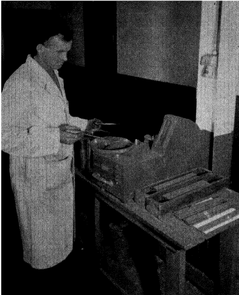
A , accurate weighing of the carbide powder for each briquette; molded bars are in foreground.
