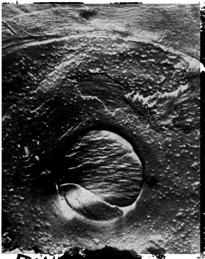
Fig. 3. The surface of an undercooked pine tracheid at a bordered pit showing the lignin sheath and underlying primary fibrillar structure. Note the spot where the lignin sheath is mechanically broken. No description of the membrane under the pit aperture has been advanced (Horio, Kobayashi, and Komagata 10 ). Magnification \times 7,500 .
