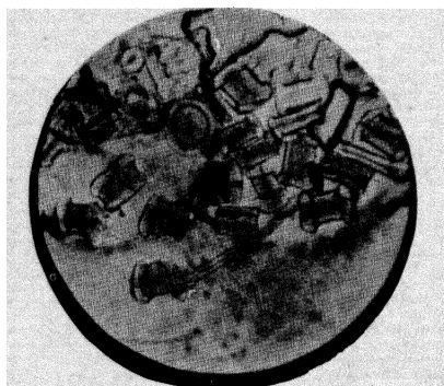
Fig. 45 Photograph showing the "dumbbell-like" swelling of microscopic sections of cotton fibers in mercerizing solutions (Willows and Alexander 39 ).
