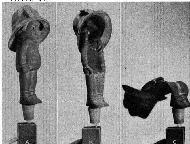
The india-rubber figure collapses when connected to the vacuum pump.
