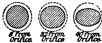
Fig. 51. Section of jet from circular orifice.
